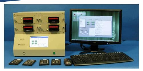
The M3100 is a full featured production Duplicator for HDD's and SSD's which copies up to 8 drives simultaneously. A front panel 7" Touch screen provides full control of the M3100. Alternatively, a LCD, keyboard and mouse using a Graphic Interface allows users to define and execute simple or complex scripts while also providing network connectivity.
