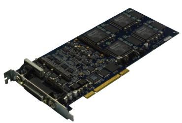
Featuring four independent output channels for YPbPr, RGB, S-video, or Composite output, and AC-3 audio, the Harmony 4ES PCI Card delivers industrial-strength MPEG-2 decoding. With this board, you can operate multiple boards in one server, integrate high-quality video and graphics with transparency, and reduce the cost per channel in multi-channel systems.
