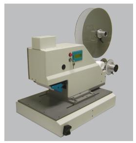
The AccuPlace model 3065 is designed to assemble virtually any self-adhesive component within its 3.0" x 6.5" / 7.6 cm x 16.5 cm capacity. The machine has a compact foot print and offers a wide range of features, options and software parameters. This allows optimal adaptation to your specific requirements. Various placement actuator options allow practically any kind of part placement. The model 3065 is the most capable and accurate machine of its kind.
